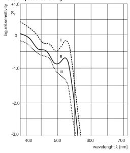
The values stated show the densities of 0.5 (I), 1,0 (II) and 1,5 (III) measured in reflection. The sensitivity is the reciprocal of the exposure in  $(mJ/m^2)$  needed to produce the relevant densities.
