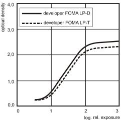
Automatic processing: processor Protec M 45 cycle 2 min/34 °C developer /fixer: FOMA LP-D/FOMAFIX <u>Manual processing</u>: developer: FOMA LP-T 5 min/20°C
