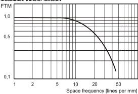
Resolving power 120 lines per mm (processing according to ISO 7829)
