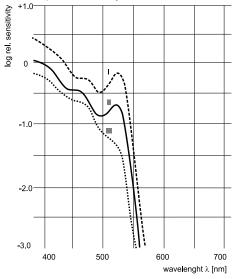
The values stated show the densities of 0.5 (I), 1,0 (II) and 1,5 (III) measured in reflection. The sensitivity is the reciprocal of the exposure in  $(mJ/m^2)$  needed to produce the relevant densities.
